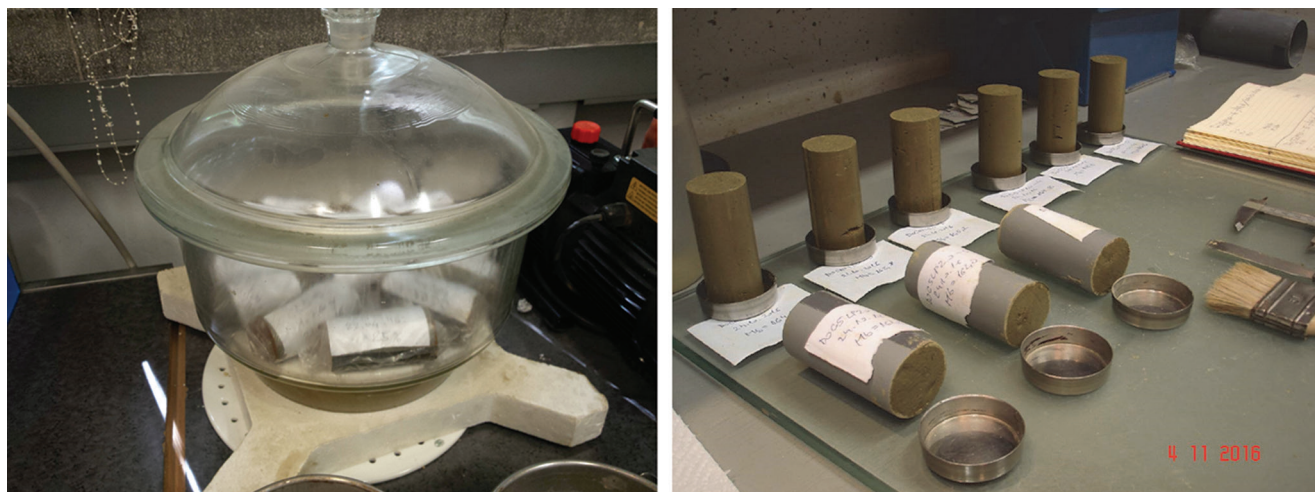
Figure 2. Keeping composite samples in desiccator and preparations for testing
