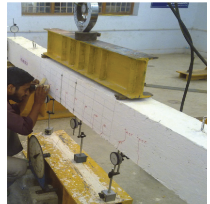
Figure 4. Crack-width measurement in progress
